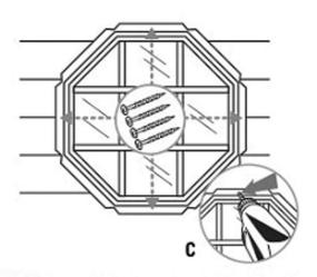
STEP 3. Secure window into opening with installation flange using pan head screws through pre-drilled holes. (Fig C)
