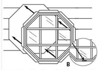
STEP 2. Drop window into opening (Make sure weep slots are to the OUTSIDE and BOTTOM). (Fig B)
